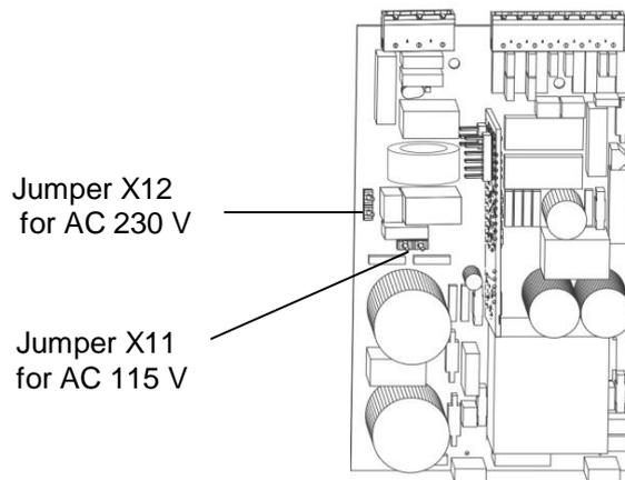
Step 3: Mark AC 115 V with 'x' and AC 230 V with '-----' on the label as indicated below.
