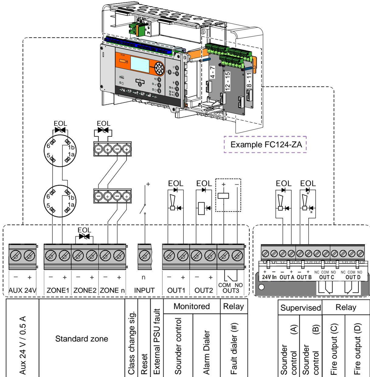
(#) 'Fault dialer' contact is open as long as the panel is in fault condition.
