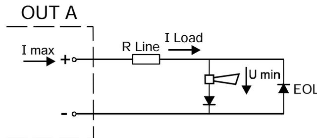
Procedure for determining the maximum available device current ( $I_{\text{Load}}$ ):
