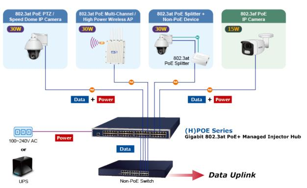
Figure 2-2-3: Network application installation
