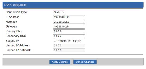
Figure 4-2-2: LAN Configuration Setup Web Page
