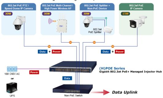
With data and Power over Ethernet from one unit, the PoE+ Managed Injector Hub series can reduce power cable deployment and eliminate the need for dedicated electrical outlets on the wall, ceiling or any unreachable place.
