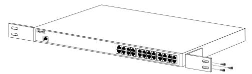
Figure 2-2-1: Brackets attaching to the PoE+ Managed Injector Hub
