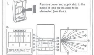
Example :ZONE "a" can be eliminated by masking the lens at area "a" (see illus.).
