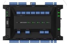
The access controller supports web configuration, which is no need to install software on a PC. By connecting with access modules via RS-485, it can extend to control up to 126 doors, which is suitable for the scenarios of subways, airports, banks, large groups and other industry projects.
