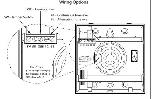
There are five terminals for the connection of wires as shown above. To activate either the alternating or continuous sound, connect a negative to the common negative terminal (GND) and connect a positive to the appropriate positive terminal (#1 or #2). To stop the sound, remove the positive or negative supply.
