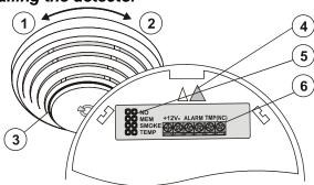
Fig. 6: 1– detector cover opening; 2 – detector cover closing; 3 – optical status signalling; 4 – arrow showing where to insert the detector; 5 – configuration jumpers; 6 – connection terminals;
