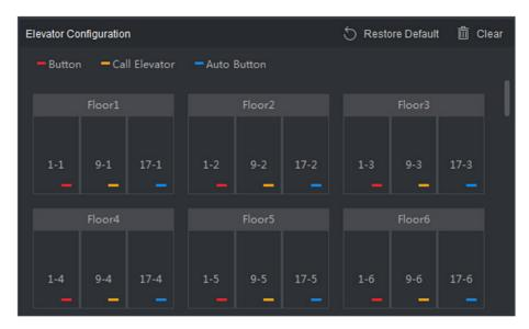
Figure 15-11 Relationship between Relay and Floor
