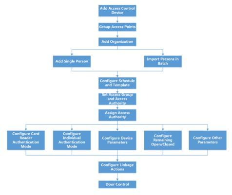
Figure 15-1 Flow Chart of Access Control
